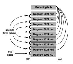
Figure 2.3.2b: SRC cables segment a managed stack for connection to switching hub ports.
